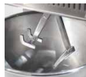
Braccia inox smontabili Removable stainless steel arms
